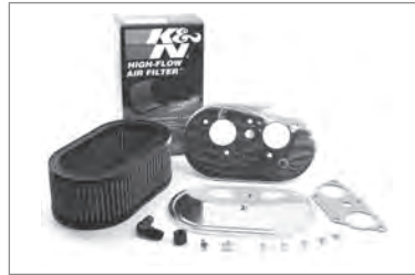
K&N Air filter Solex 40 P11-4 carbs for 356SC, Super 90 and 912 NLA.100.500.00
