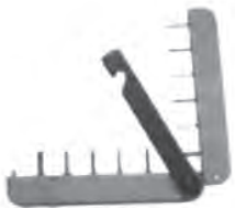
Plug Gap Check Gauge Original Bosch spark plug Gap checking tool NLA.721.681.00
