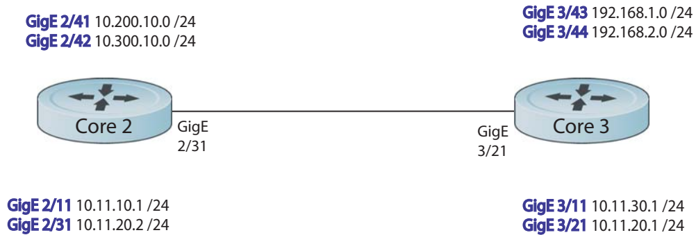
Figure 389 RIP Topology Example
